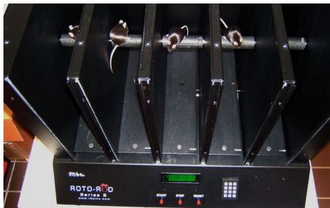
Fig. 3. Mice being tested on a Rotarod.
