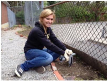
Figure 3. Testing the soil for lead with the XRF analyzer.
